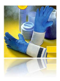
Contact or exposure to cryogenic materials or the containers in which they are held can cause injury. Skin contact with a low temperature material can produce a cold burn
